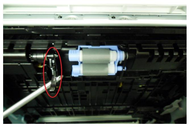
The original service manual does not list a part number for this but a service bulletin was released showing the repair procedure and part number for the flag RM2-5375.
